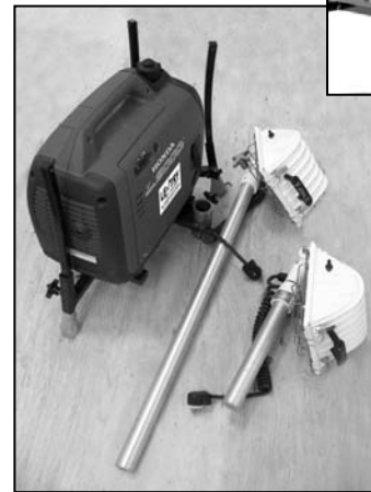
Figure 7: Dual unit with lights disconnected
